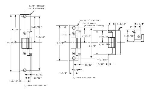
Solenoid power requirements; 12VDC, 0.38 A, 24 VDC, 0.19 A
